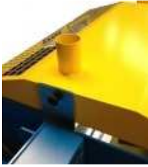
Extraction point for smoke and dust
