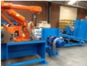
Last year we informed you about the possibilities of [automatic sorting](#). Now you can also see our solution for automatic dismantling of pallets. It's the way for fast, save and more accurately removal of broken parts, with a robot. After dismantling, the pallet can be repaired directly. Curious how this works? See the next article.
